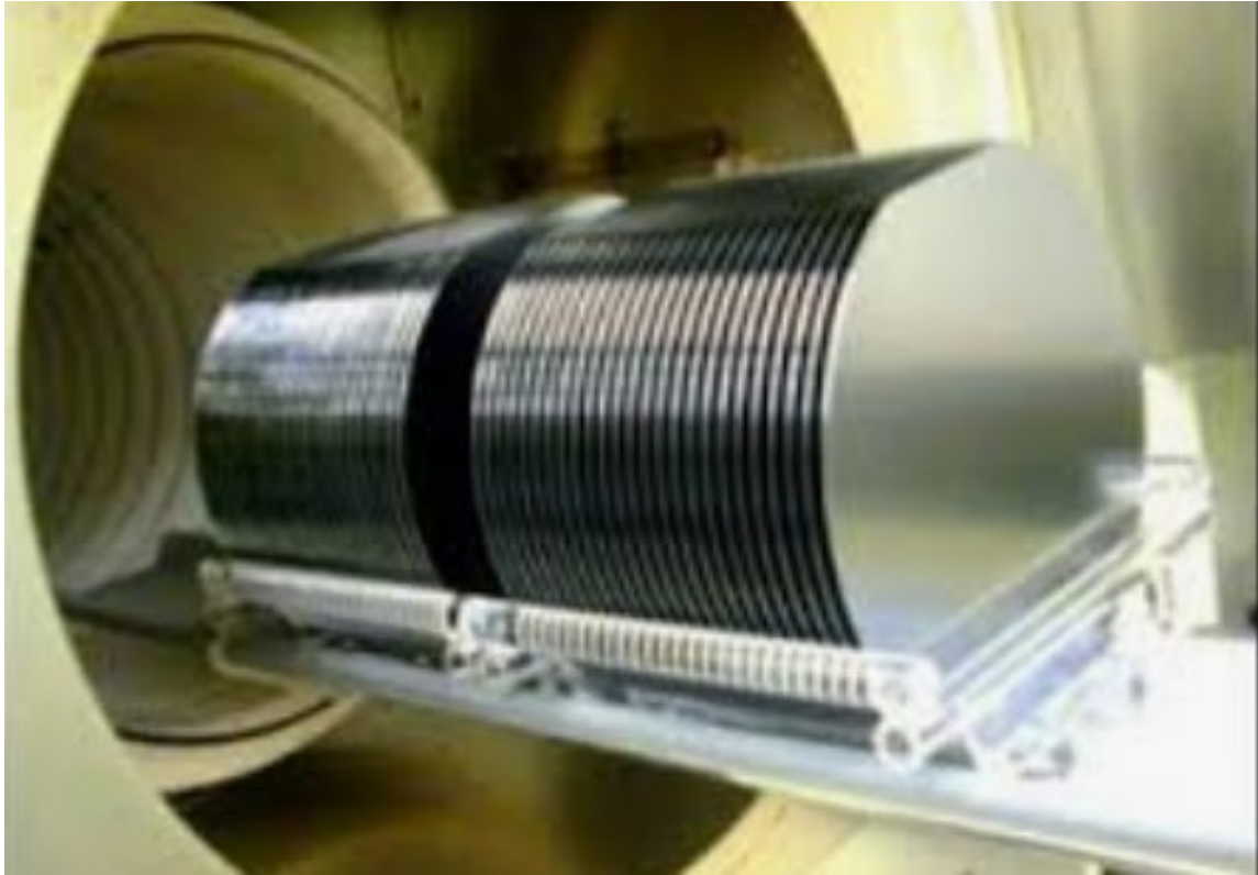
300mm wafers loading in diffusion furnace
